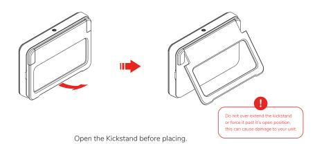
Kickstand will stop at open position. With kickstand open, the radar will be at the correct tilt angle on a flat surface.
